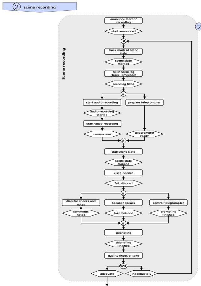
Figure 5: Detailed process component ‘Scene recording’
